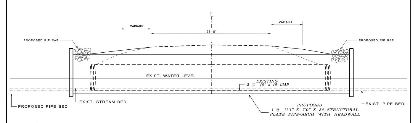
NOTES: \* PROPOSED 1 @ 11'1" X 7' X 54' STRUCTURAL PLATE ARCH PIPE WITH HEADWALLS TO BE BURIED 1' BELOW EXISTING STREAM BED
