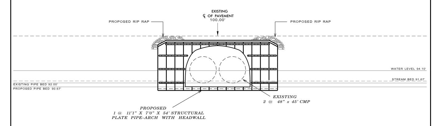
NOTES: \* PROPOSED 1 @ 11'1" X 7' X 54' STRUCTURAL PLATE ARCH PIPE WITH HEADWALLS TO BE BURIED 1' BELOW EXISTING STREAM BED
